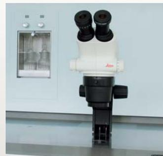
Fig.1: The classical Greenough stereomicroscope Leica S6 E with 6.3:1 zoom and standard magnification of 6.3x-40x has a comfortable 38° viewing angle. The optical design coupled with this ergonomic viewing position allows this microscope to be used for long periods without causing eye strain. Courtesy of: Dr. B. Keppi, Laboratoire de PMA, Beaumont, France
